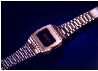
The Hamilton Pulsar: the first LED (light-emitting diode) digital wristwatch. The time was displayed at the touch of a button.
