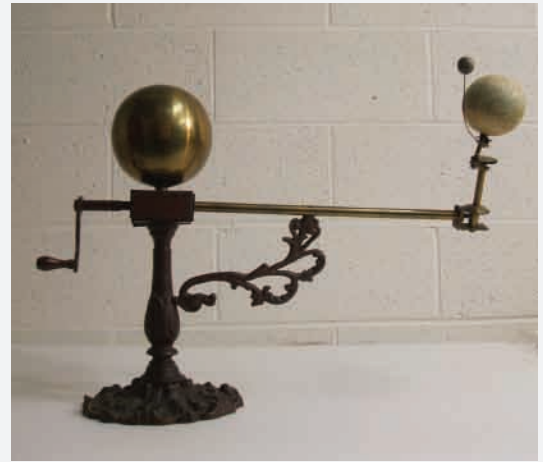
a tellurion from the mid-1800s, used to model the movements of the sun, moon, and earth
